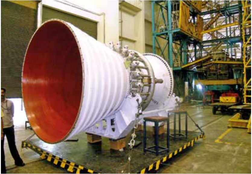
35. SITVC for PSLV first stage with twenty-four single pintle electromechanical injection valves, equispaced around nozzle
