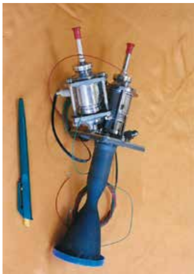
45. AOCS Thruster of 10N thrust
