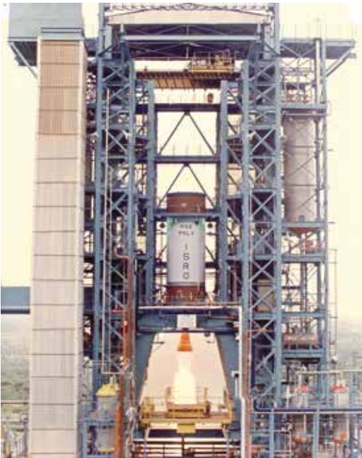
52. Principal test stand to test high thrust liquid engine, stage and turbo pumps. PSLV second stage is under test
