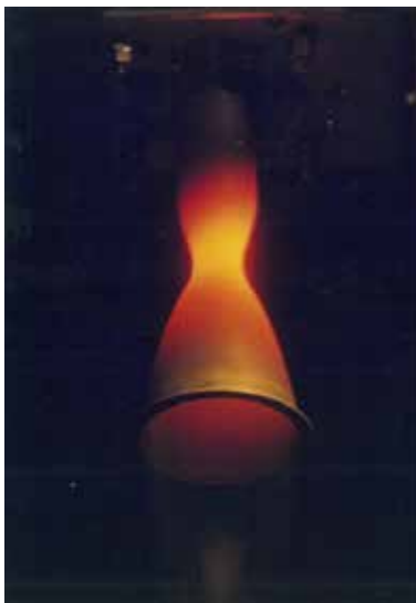
44. Long duration high altitude simulation test of 22N AOCS Thruster in vacuum chamber
