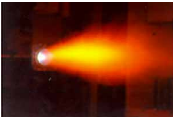
47. First successful static test for 50 seconds duration of 12-tonne thrust cryogenic engine in 1998 at Mahendragiri
