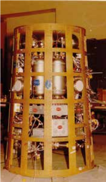
31. Bi-propellant Reaction Control System (RCS) for the second stage of SLV 3 and ASLV
