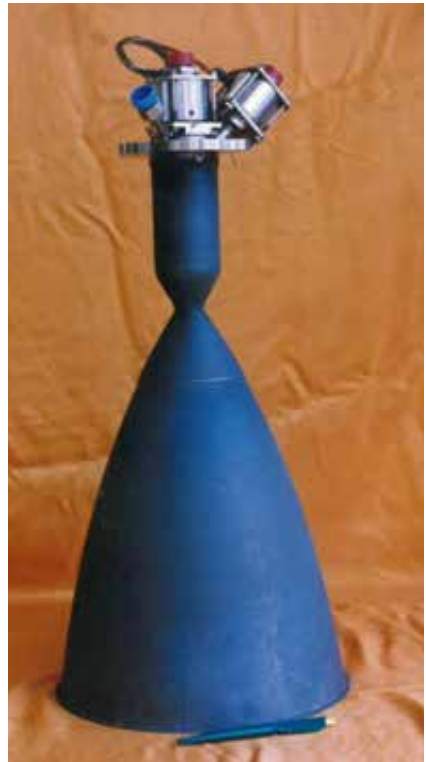
43. Attitude and Orbit Control System (AOCS) Thruster of 22N thrust
