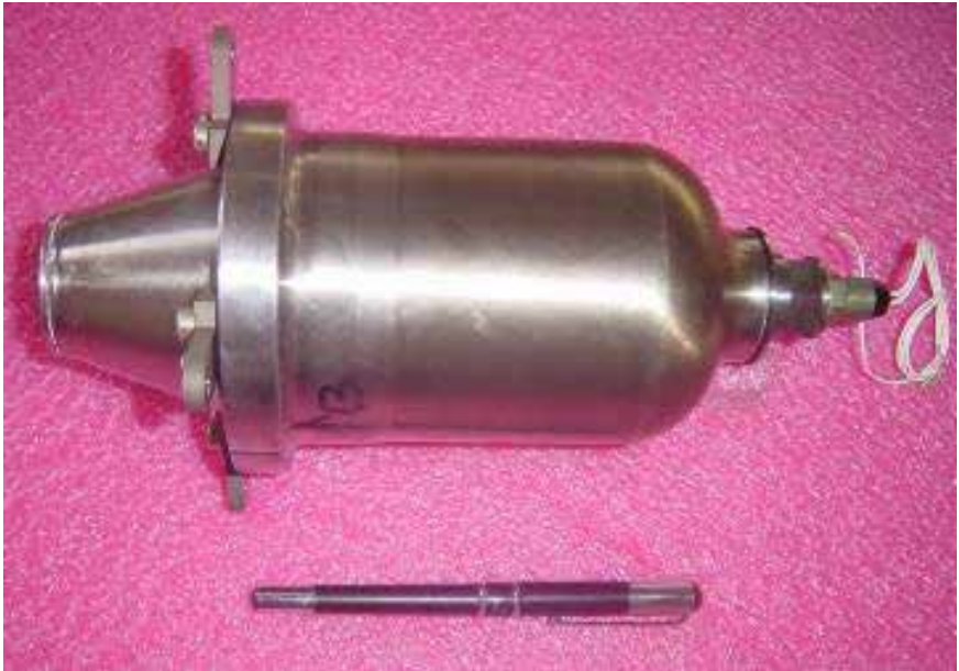
26. De-spin Motor: Special purpose small solid motor for Chandrayaan 1 mission
