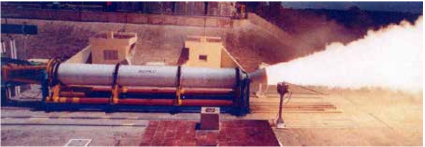
24. Static test of PSLV strap-on motor PS0 at STEX, SDSC
