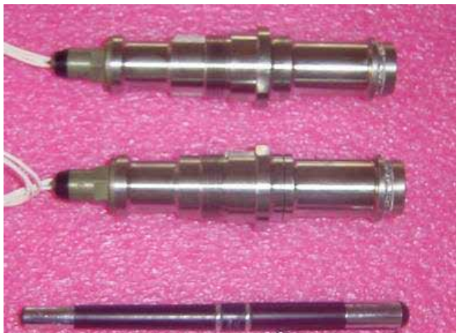
25. Spin Motor: Special purpose small solid motor for Chandrayaan 1 mission
