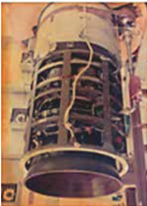
33. Secondary Injection Thrust Vector Control (SITVC) system for the first stage of SLV 3 and ASLV
