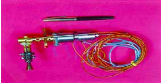
38. 1N Mono-propellant thruster for IRS
