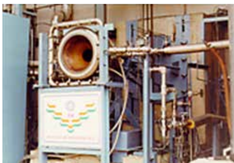
46. First regeneratively cooled thrust chamber of 12 tonne thrust cryogenic engine with Liquid Oxygen-Liquid Hydrogen propellants, assembled on the test bed at Mahendragiri
