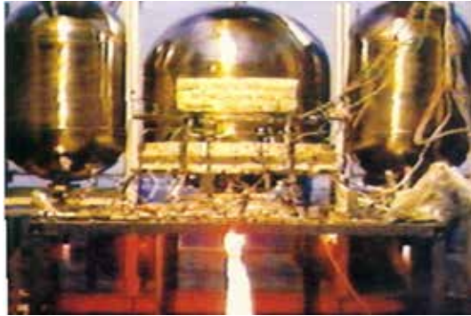
41. INSAT Propulsion System with Liquid Apogee Motor (LAM) firing
