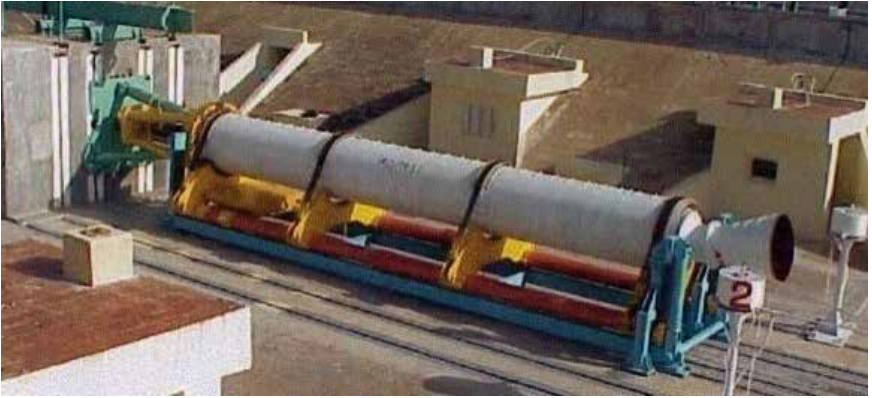
23. PSLV strap-on motor PS0 with canted nozzle on test bed at STEX, SDSC
