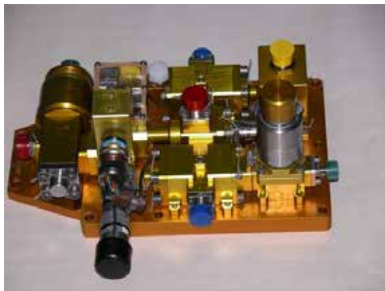
49. Pressurization Module- Group I for PSLV first stage reaction control system RCS) and fourth stage
