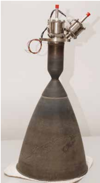
42. Liquid Apogee Motor (LAM) of 440N thrust
